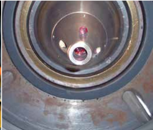
Light sensors for automatic center recognition
