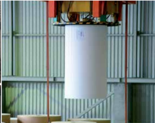
Automatic recognition of paper-unwrapping during the transport
