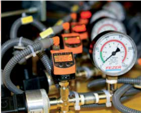
Analysis of each suction chamber's vacuum level by digital vacuum switch
