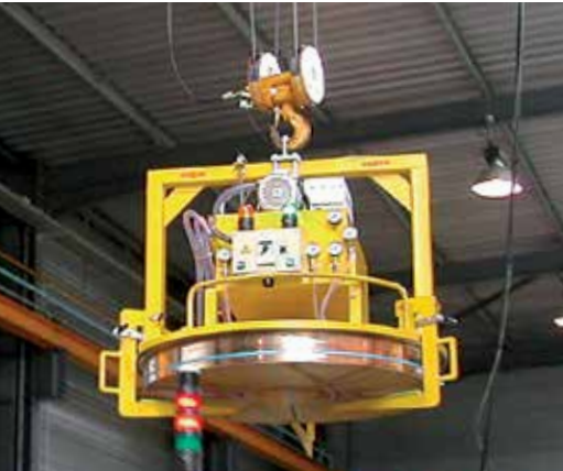
Mechanical undergrippers for long transport ways over work areas
